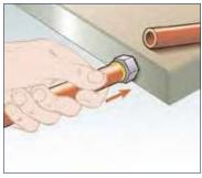
2. Insert fitting into hose until first barb is in hose. Place end of fitting against a flat object (bench, door, wall) and grip hose approximately 1" from end and push with a steady force until end of hose is covered by yellow plastic collar. Alternatively please use the Parker Assembly Tool No. 611050G or 611050HV.
